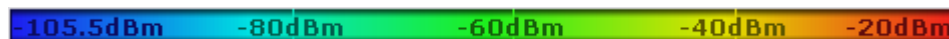
Fig. 6-11: Linear color curve shape = 0; colors are distributed evenly over the complete result range
